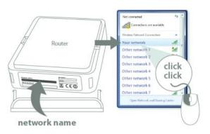
• Push the OPS Button on the router. For 2.4GHz, press 0-5 seconds. For 5GHz, press 5-10 seconds.
