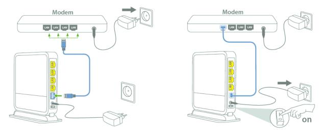
Connect the supplied power-adapter to the power inlet port and connect it to a wall outlet. Switch the router on by flipping the switch on the back of the device. The router automatically enters the self-test phase. During self-test phase, the Power LED will be lit continuously to indicate that this product is in normal operation.
